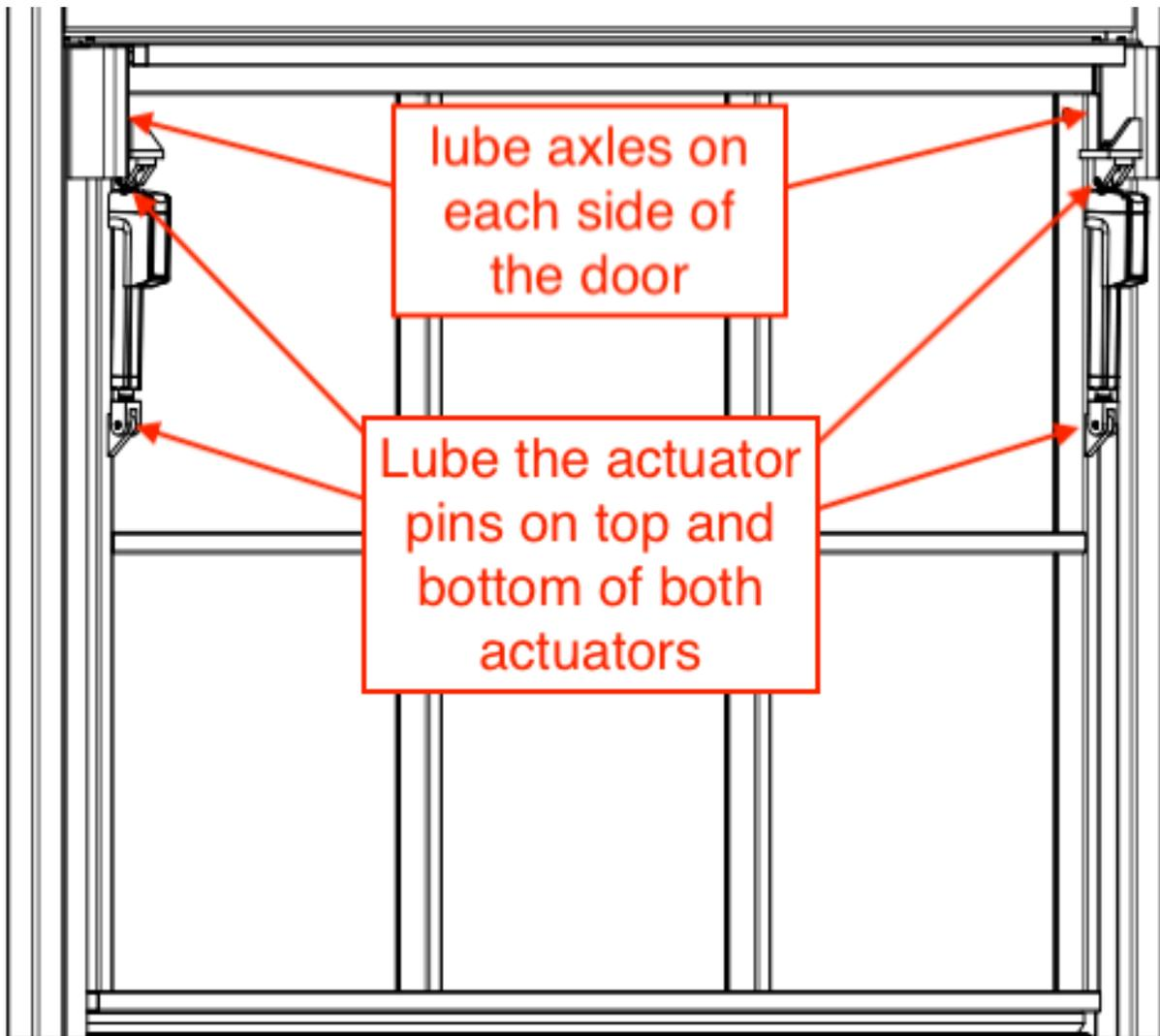
Above is a diagram of the door and the lubrication points on your door system.
